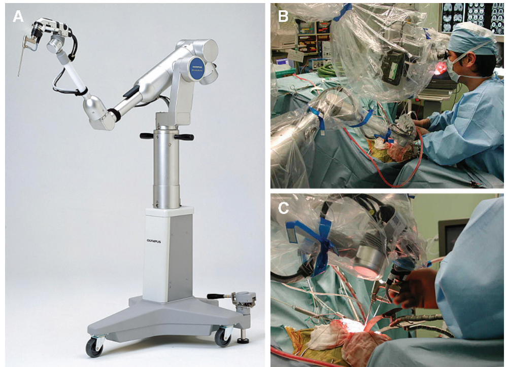
FIGURE 1. A, an endoscope-integrating holding device (EndoArm; Olympus). B, operative view of the microscope, endoscope, and monitor. C, joint motion is controlled with high-pressure gas and low force. It can be fixed with 1-touch operation, providing superior safety and handling.
